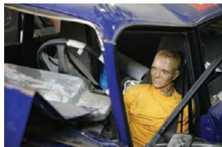
FIG. 1.22 Dummy used to measure the effects of car impacts.
