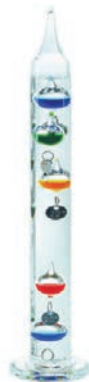
FIG. 3.19 Galileo's thermometer , which is in fact a thermoscope , “measures” the temperature in the environment.
