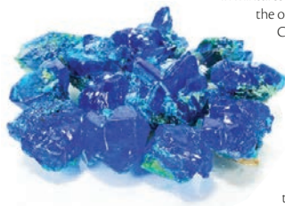
FIG. 1.52 Copper sulfate II ( \text{CuSO}_4 ) crystals obtained from an aqueous solution by crystallization.
