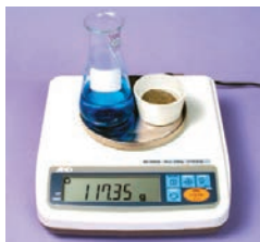
FIG. 1.45 To express the mass concentration of a solution, it is necessary to measure the mass of the solute and the solution.
