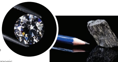
FIG. 2.52 Graphite and diamond may seem as totally unrelated materials, but, because of their characteristics, they are similar. They are both formed by the same type of atom but have different crystalline structures.
