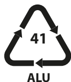
FIG. 2.23 A triangle made out of arrows is the international recycling symbol, if an object has it, then it can be recycled. This symbol also contains codes, number 41 and the letters ALU indicate it is an product made of aluminum.
