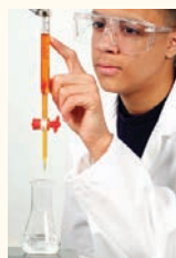
FIG. 4.9 Burettes are the correct instruments to make a titration.
