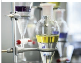
FIG. 1.50 Separation funnel ready to be used.
