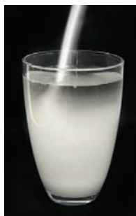
FIG. 1.38 Saturated sodium chloride solution in water. If heated, more salt will dissolve.
