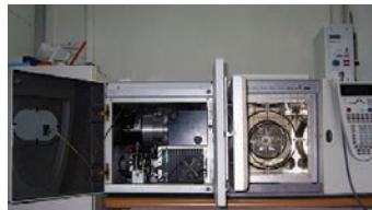
FIG. 1.55 To identify unknown substances, chemists use various techniques and devices like the gas spectrometer. This picture shows part of the equipment to identify semi-volatile organic compounds at the National Institute of Ecology.
