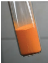
FIG. 1.65 Mercury (Hg) is a silvery-white liquid metal, while the mercury oxide (HgO) is a brick-red powder.
