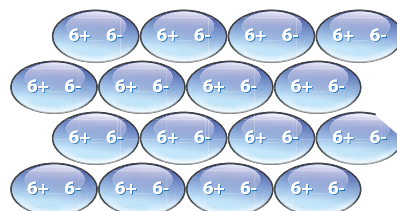
FIG. 2.50 In a solid polar molecule, molecules are arranged according to the interactions of dipoles that form them.
