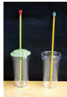
FIG. 3.16 Both jars have a thermometer, one jar is covered to simulate a closed "atmosphere", and the other one is not.
